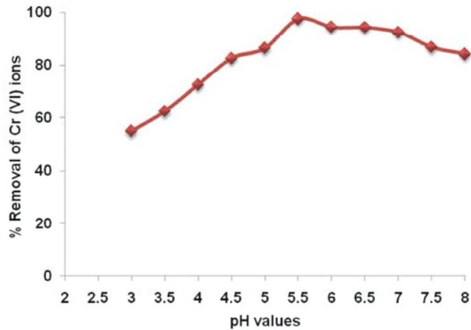
Fig. 3: Effect of pH on Cr (VI) removal
