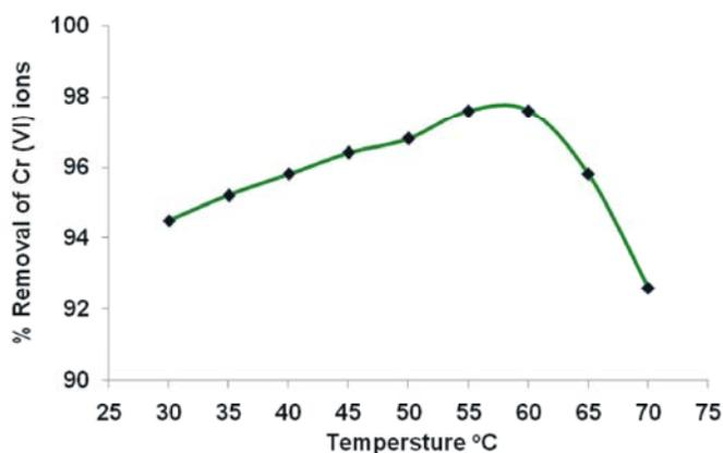
Fig. 7: Effect of temperature on Cr (VI) removal
