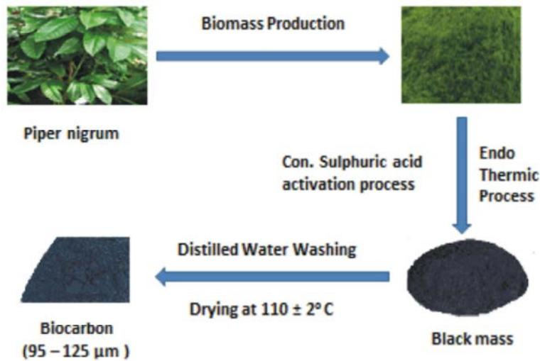
Fig. 1: Process for the preparation of biocarbon
