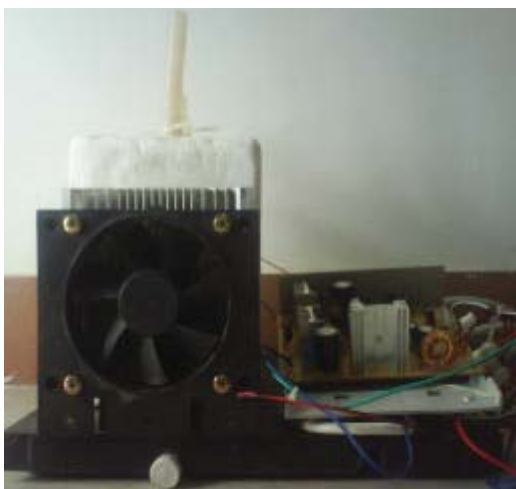
Fig. 3: A picture of the built water condensation system
