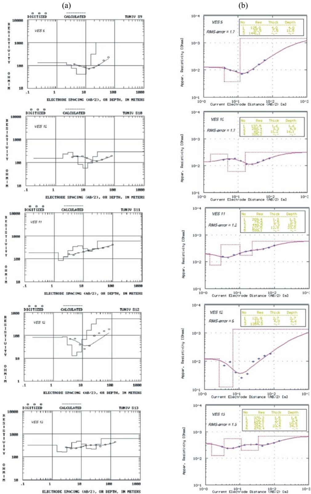
Fig. 5: (a) VES's multi-layer models using Ato program [7] and (b) the layering models using Resist [8]
