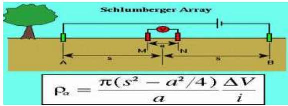
Fig. 3: Sketch diagram shows the Schlumberger electrode arrays
