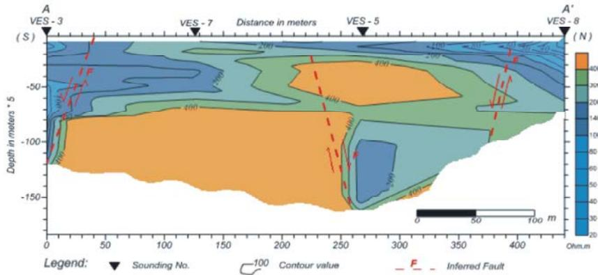
Fig. 6: Subsurface true resistivity contour section (A-A') through VES's 3, 7, 5 and 8
