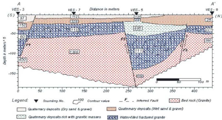
Fig. 7: Geoelectric section (A-A') passing through VES's 3, 7, 5 and 8
