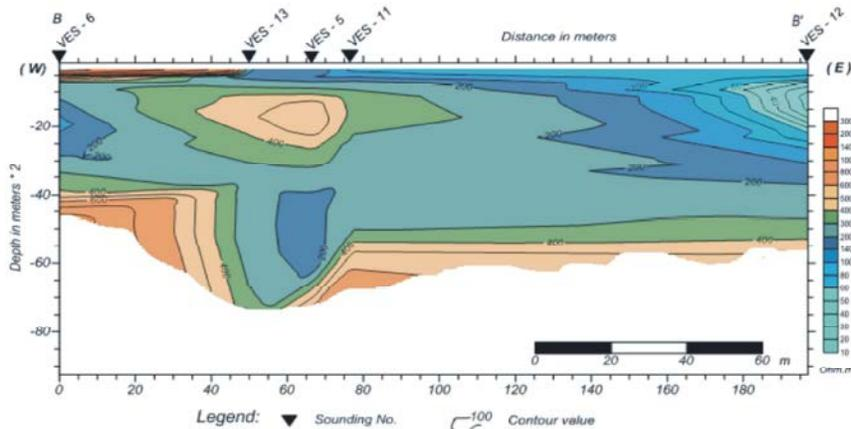
Fig. 8: Subsurface true resistivity contour section (B-B') through VES's 6, 13, 5, 11 and 12
