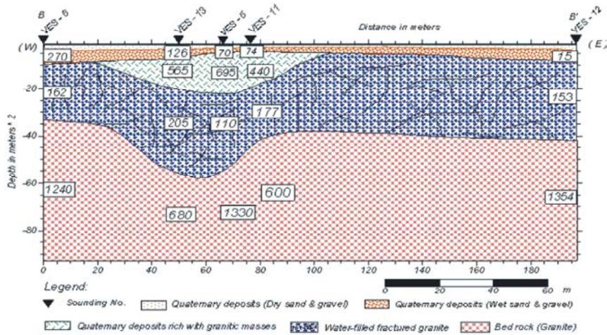
Fig. 9: Geoelectric section (B-B') passing through VES's 6, 13, 5, 11 and 12
