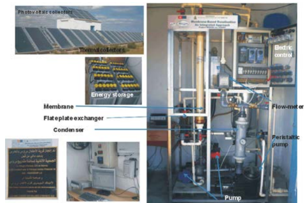
Fig. 2: Photo of the pilot plant solar VMD
