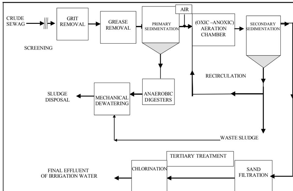
Fig. 2: Schematic of the Wastewater Treatment Plant at Al Hofuf, Saudi Arabia.
