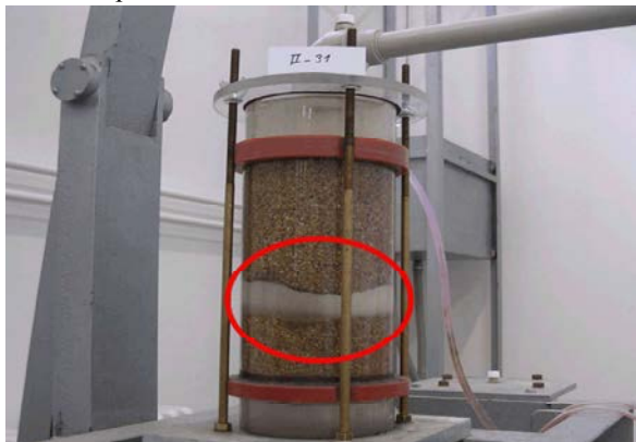
Fig. 8: The finishing by complete total collapse
