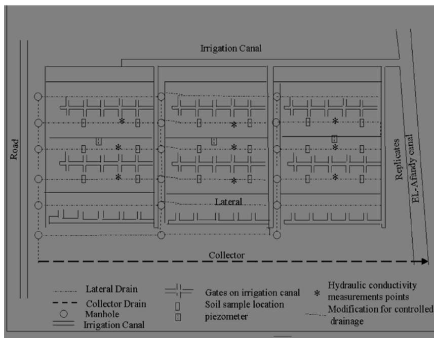
Fig. 1: Schematic Diagram of Zankalon Experimental Station
